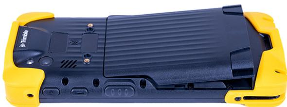
2. Press in and hold the two plastic clips at the end of the battery, then push the battery forward and down into the battery compartment.
