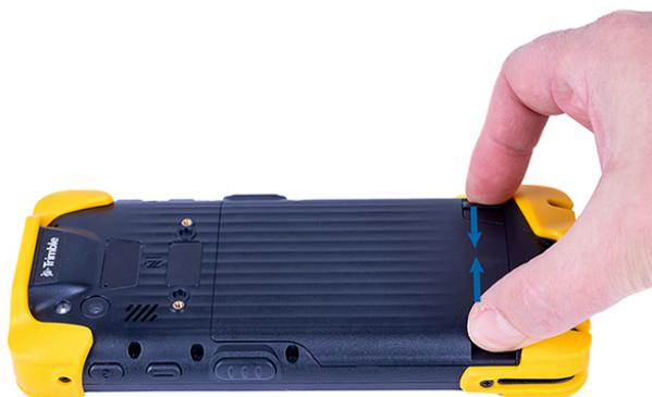
2. Push the battery forward and lift to remove it.
