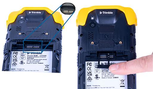
The card holder can hold two nanoSIM cards, or one nanoSIM card and one microSD card at a time. Insert your cards as needed, as follows:
