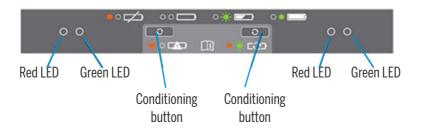
Figure 2.6 Dual Slot Charger control panel
