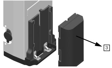
Figure 5.23 Removing battery from external radio
