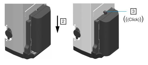
Figure 5.21 Fitting battery to external radio
