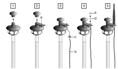
Figure 5.24 Fitting the antenna extension kit.
