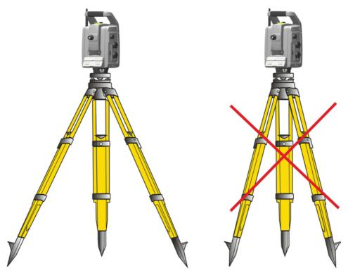
Figure 3.1 Correct instrument set up
