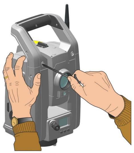
Figure 2.13 Removing the instrument handle
