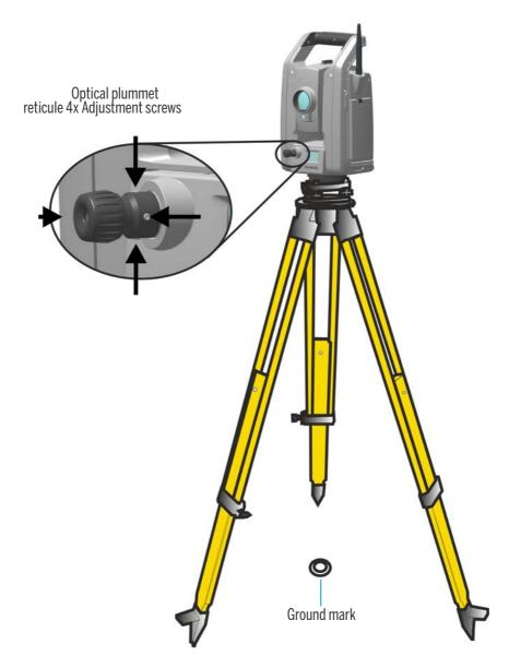
Figure 3.11 Optical plummet adjustment
