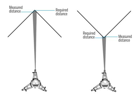
Figure 4.3 Measuring to an inner and an outer corner
