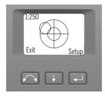
Figure 2.11 Electronic leveling screen on the face 2 display
