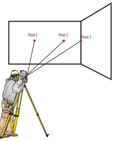
Figure 4.4 Offset measurement
