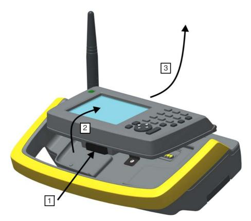
Figure 5.16 Detach Trimble CU from Trimble Robotic Holder
