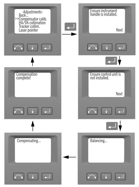
Figure 3.3 Compensator calibration routine
