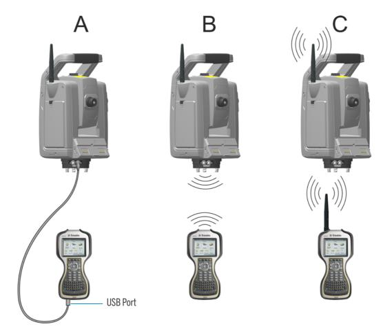
Figure 3.17 Connecting the TSC3 to the instrument
