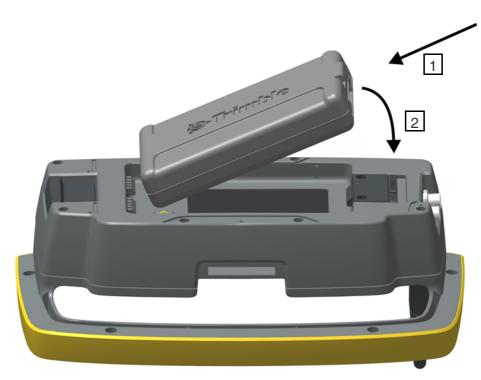
Figure 5.13 Attaching a battery to the Trimble Robotic Holder
