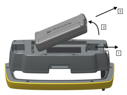
Figure 5.14 Detaching a battery from the Trimble Robotic Holder
