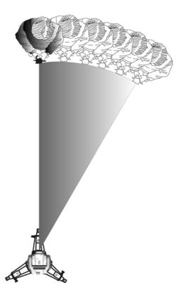
Figure 4.5 The Trimble S Series Total Station Autolock function.
