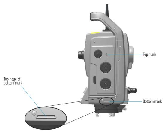
Figure 3.9 Instrument height marks
