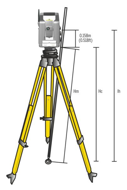
Figure 3.10 Instrument height measurement
