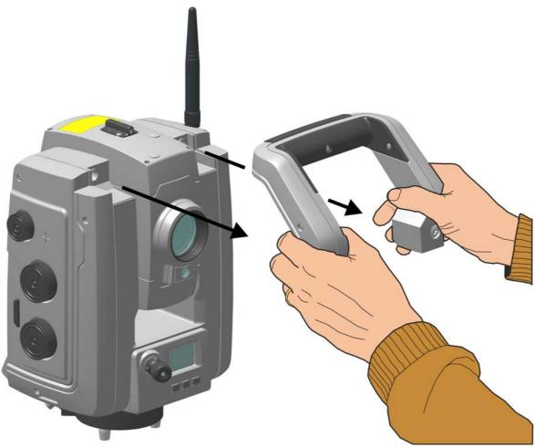
Figure 2.14 Detaching the instrument handle
