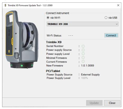
The connection to the instrument succeeds if you have previously connected to it with a Wi-Fi password.
