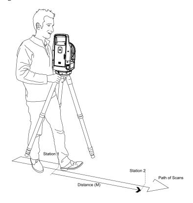
Move the tripod and the instrument from one station to the next:
