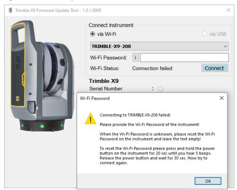
If you don't know the Wi-Fi password, leave the Wi-Fi Password field blank and press the On/Off key of the instrument for twenty seconds to reset the Wi-Fi password to the factory default value. Release the On/Off key once you hear five beeps and wait thirty seconds more before reconnecting:
