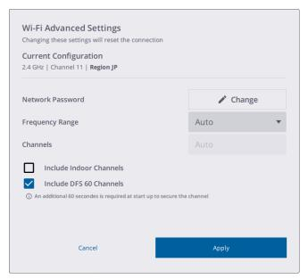
Out of the Auto mode, you can switch between **5 GHz** and **2.4 GHz**. The **5 GHz** frequency provides a faster data exchange rate at a shorter distance while the **2.4 GHz** frequency offers coverage for further distances, but may perform at a slower speed in the data exchange. Both frequencies can be used with a multitude of channels including indoor-use channels.
