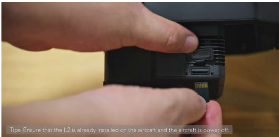
Figure: microSD card insertion
