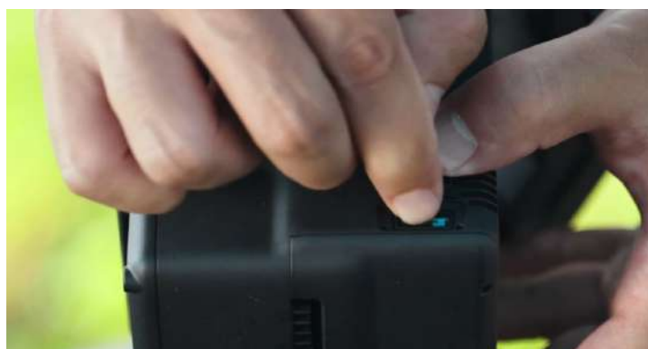
Figure: Removing the microSD card for data export after the task ends
