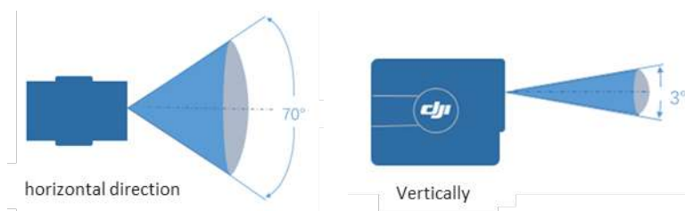
Figure: Scan angle in repetitive scanning mode
