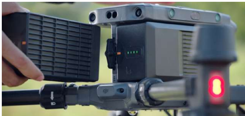
Figure: Battery hot-swapping
