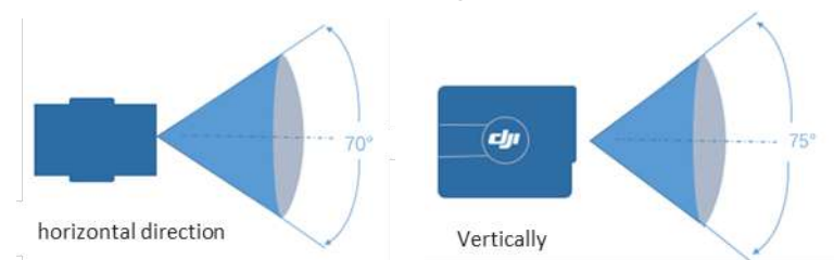
Figure: Scan angle in non-repetitive scanning mode
